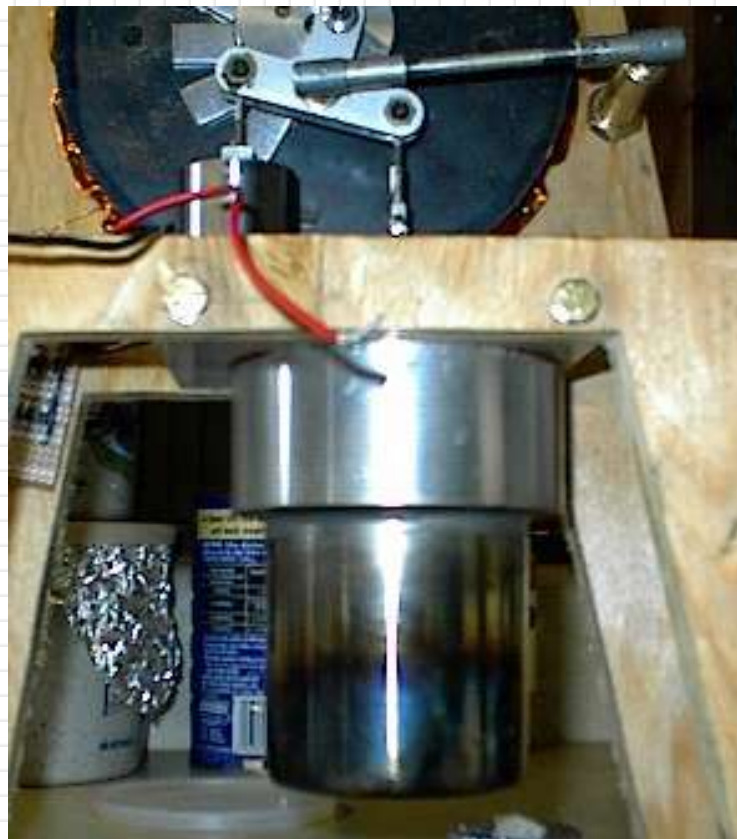
Above is the "hot end" made from a stainless steel cup and aluminum housing....
