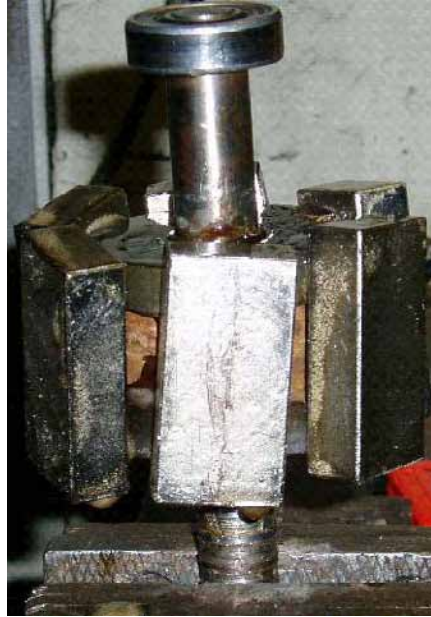
Figure 1. 40 amp car alternator rotor with magnets attached
