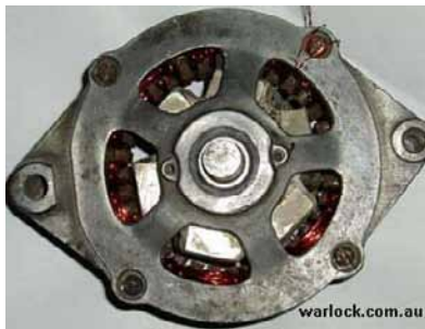
Figure 4. Completed conversion of the 40 amp car alternator
