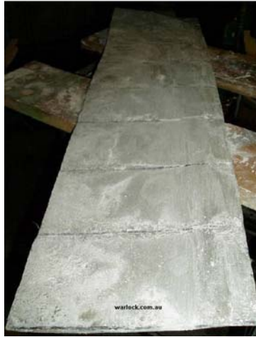
Figure 8. Positive moulds of wind turbine blades
