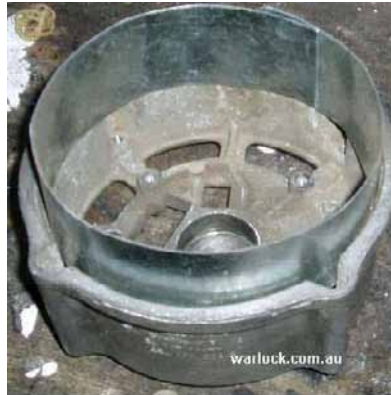
Figure 3. 40 amp car alternator stator with shielding
