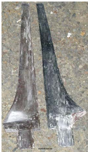
Figure 9. Negative moulds of wind turbine blades
