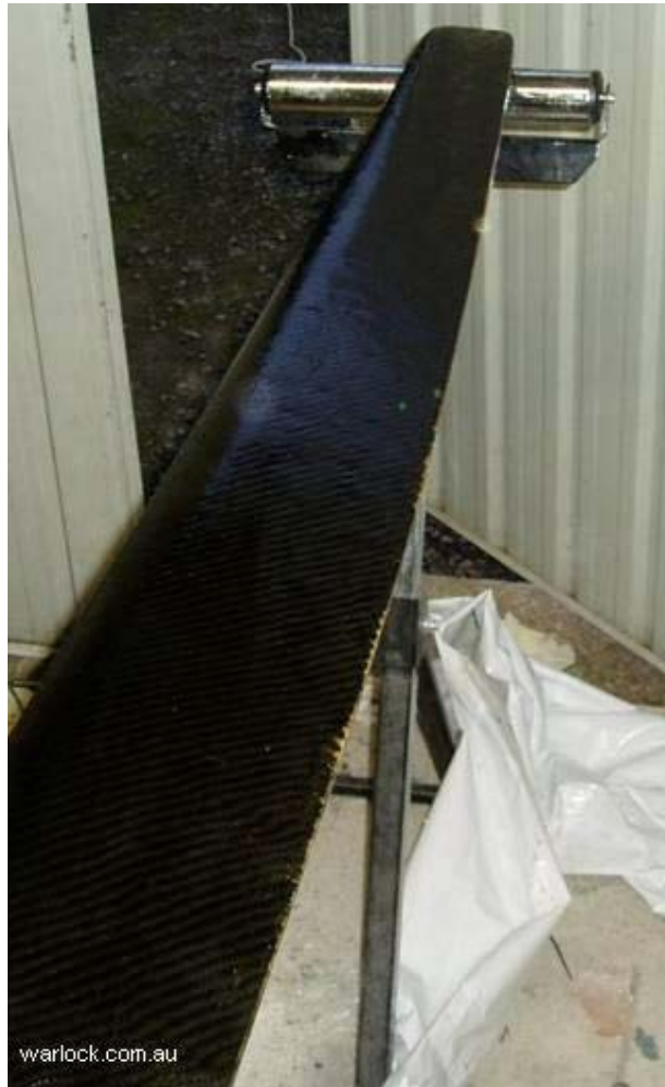
Figure 9. Blade after sanding the carbon fibre
