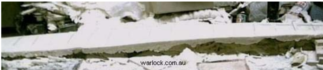
Figure 4. Skeleton filled with polyurethane foam
