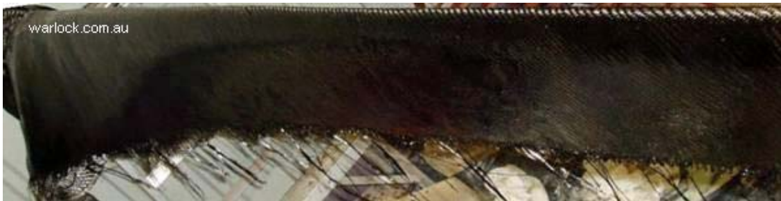
Figure 8. Blade after being covered in uni-directional carbon fibre
