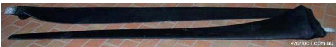
Figure 10. Completed 5m wind turbine blades
