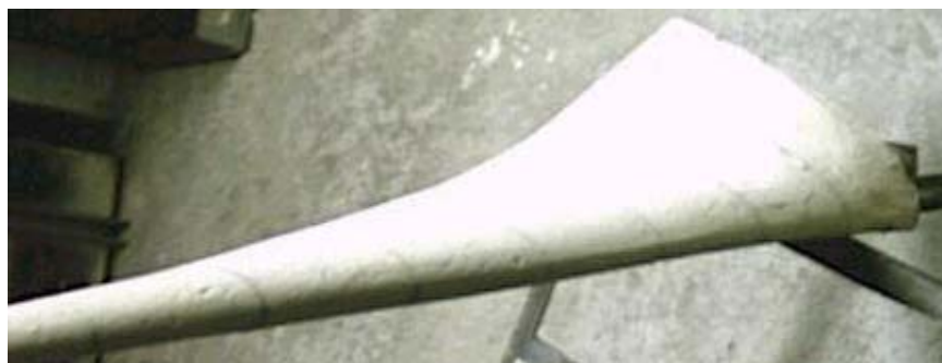
Figure 5. Polyurethane foam blade after sanding
