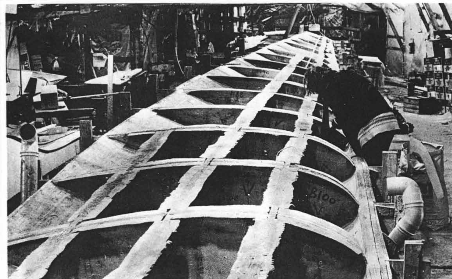
Glass-Fiber rolls being pressed down onto the mold - using a metal straight-edge.
