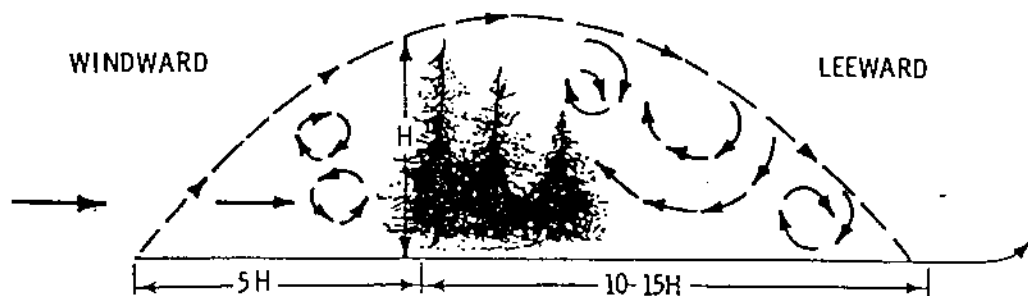
FIGURE 2. Airflow Near a Shelterbelt (Van Eimern et al., 1964)
