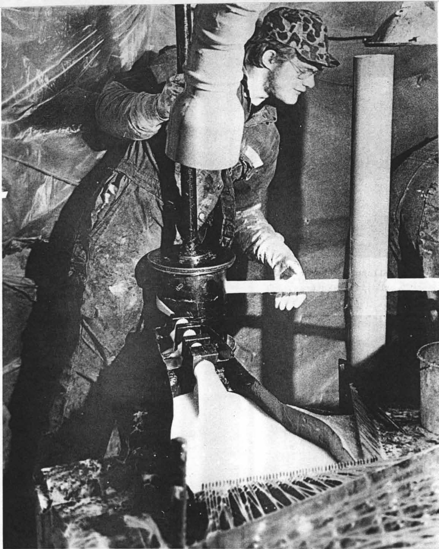
Glass-Fiber "sausage-roll" production for blades.
