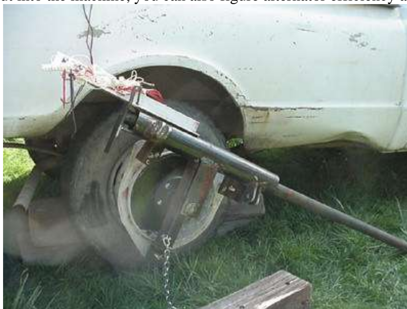
Alternator connected to wheel hub via a plywood adaptor for power testing.
