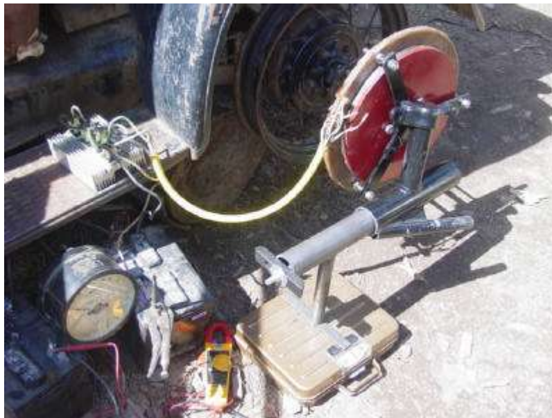
DanB's alternator dyno-testing rig
