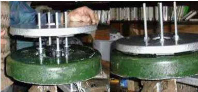
Fitting the front magnet rotor
