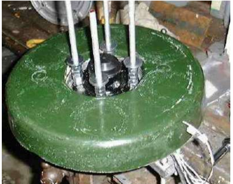
Fitting the stator
