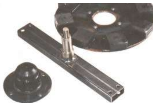
Spine, shaft, hub and magnet rotor
