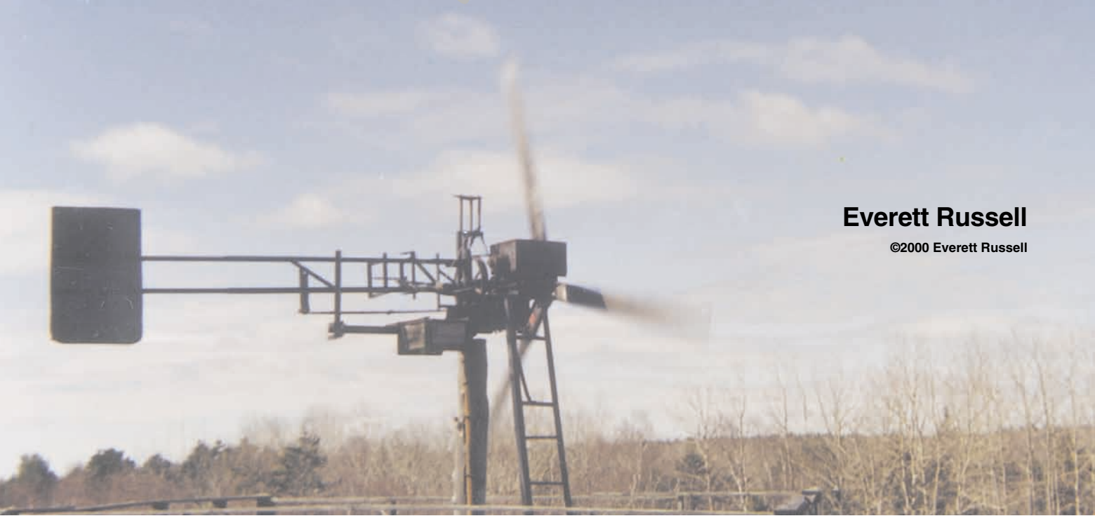
One of Everett Russell's two home-built wind generators with a 14 foot rotor diameter.
