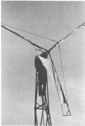
Figures 4.12–4.14. Furling the Sailwing rotor.
