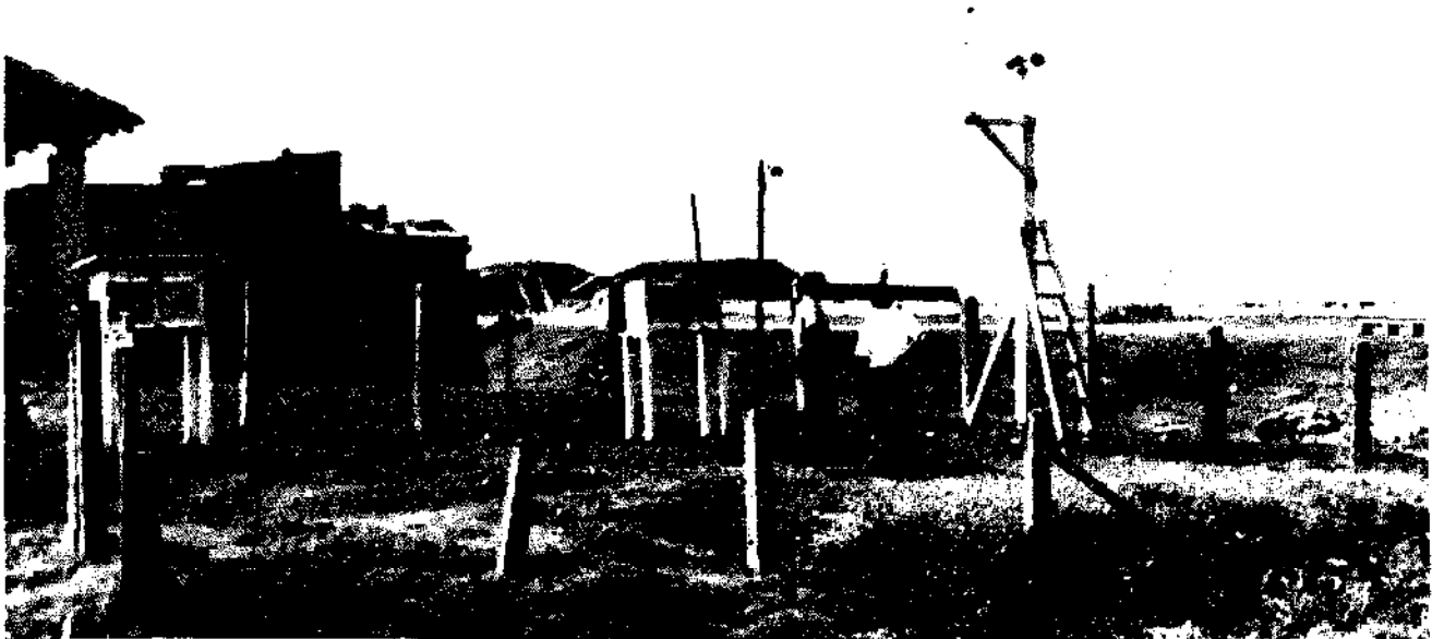
Typical example of an anemometer location that is inappropriate for data collection for wind energy applications. The anemometer is shielded off by buildings and its height above the ground is insufficient.
