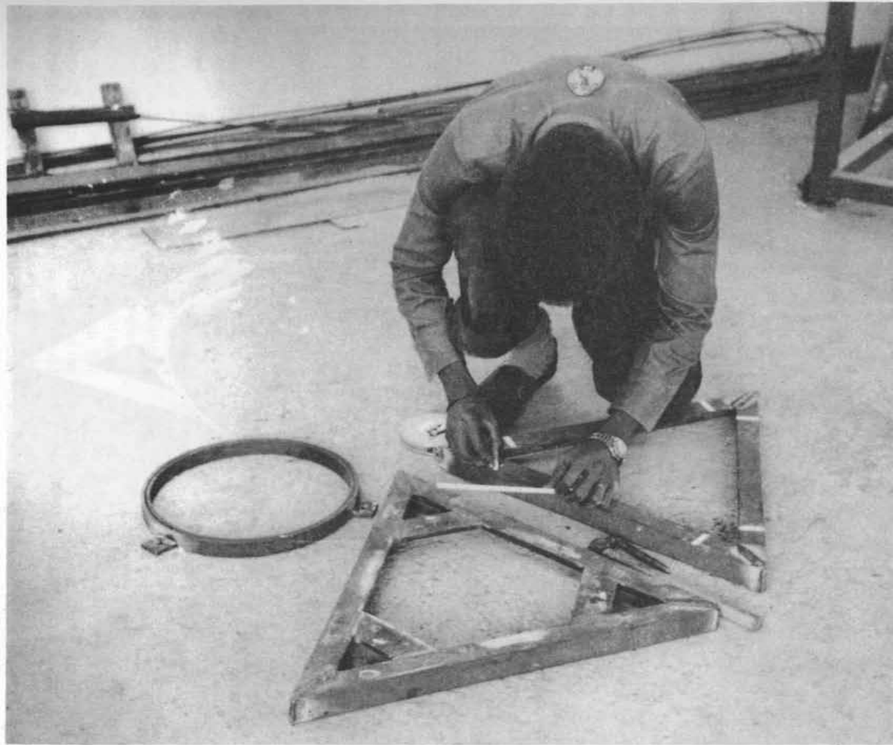
Making upper tower section frame.
