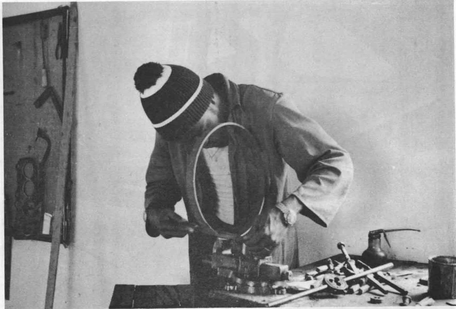
Making a turntable bearing track.
