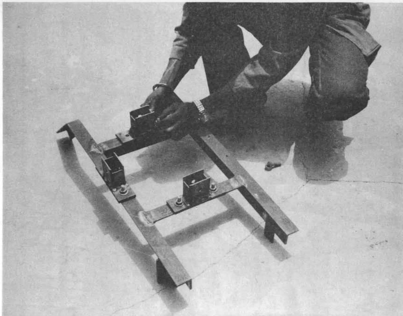
Underneath view of turntable frame showing bearing boxes.
