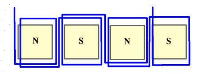
In a single phase unit the coils are wound opposite of the first. That is to say one is wound clockwise and the next is counter clockwise. If your unit has 8 magnets then it would also have 8 coils. With 3 phase you would have 3 coils for each pair
