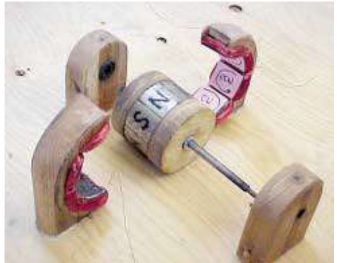
An exploded view shows the armature, stator, and pillow blocks ready to assemble into an alternator.
