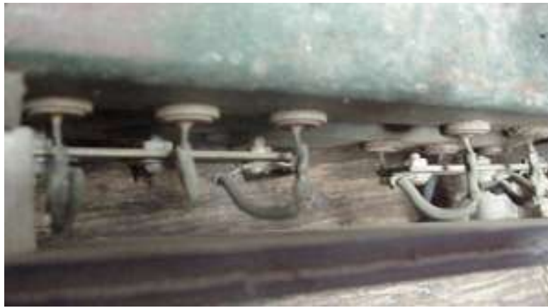
Close up of home built diode bridge
