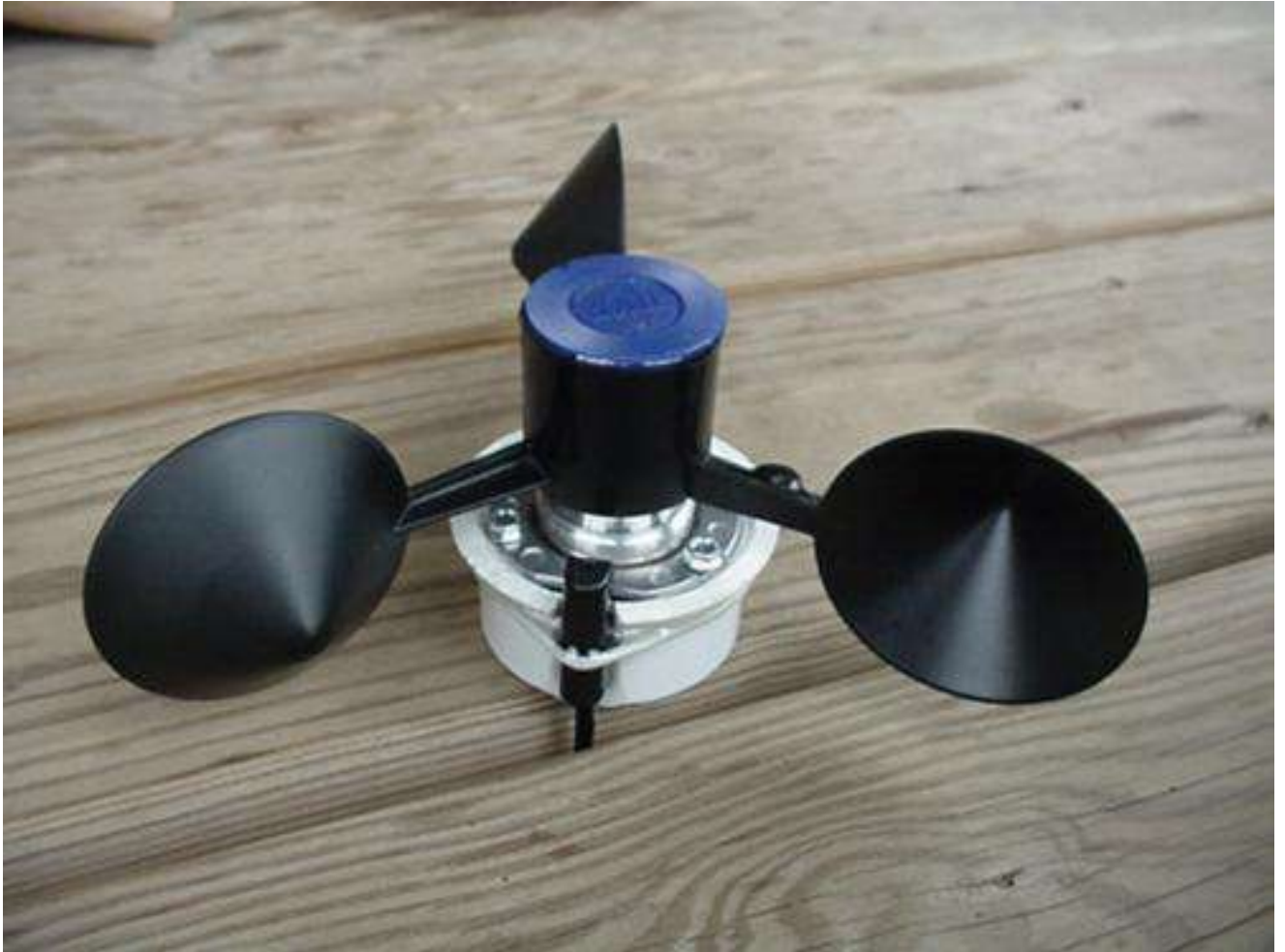
The completed anemometer cup and sensor assembly.
