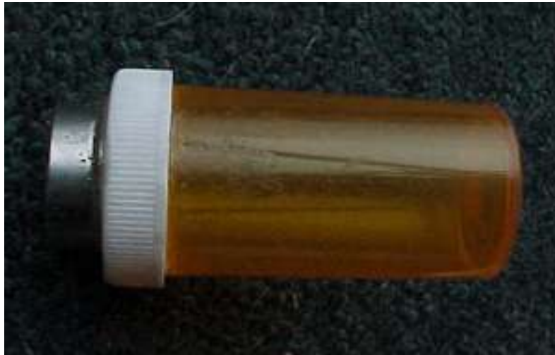
Float with magnet glued on top
