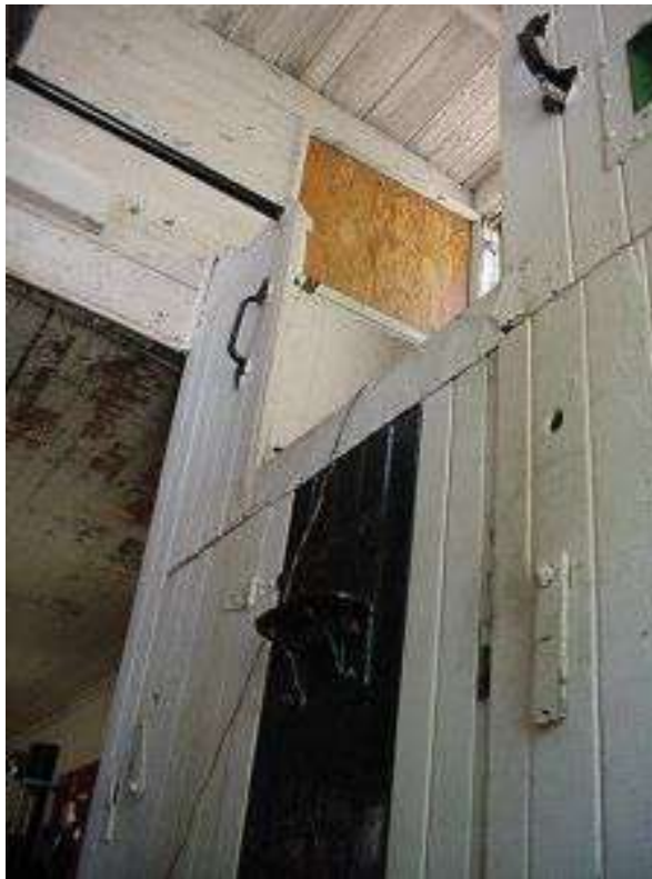
View looking up into the cupola from below. The batteries are located in the compartment underneath the cupola seats, just below the unpainted plywood panel. Note the original cabinetry, and metal step bracket!
