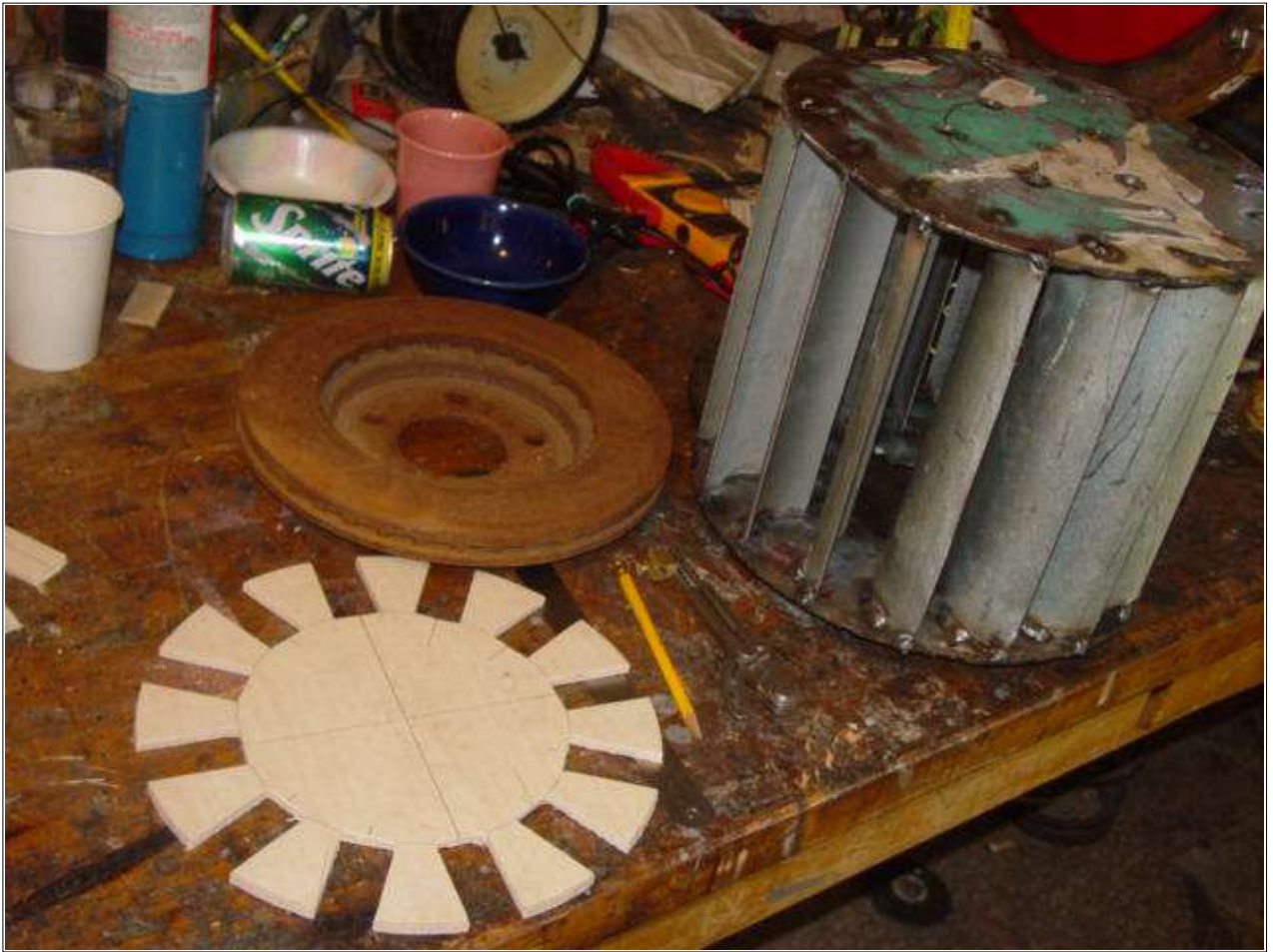
I made a template from plywood to make positioning the magnets on the brake rotors easy. Pictured above is the template, and one brake rotor.
