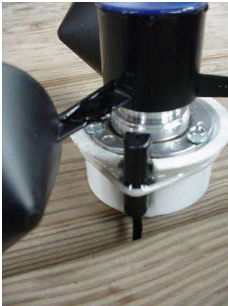
Completed anemometer hub assembly, mounted in PVC reducer, with sensor attached.
