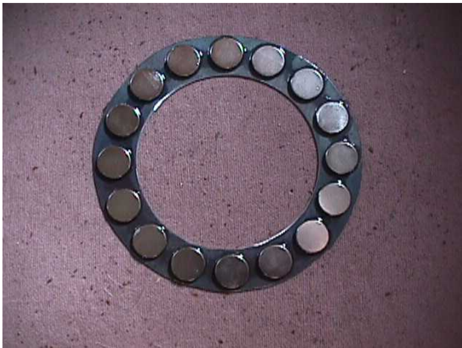
Magnets mounted on steel ring
