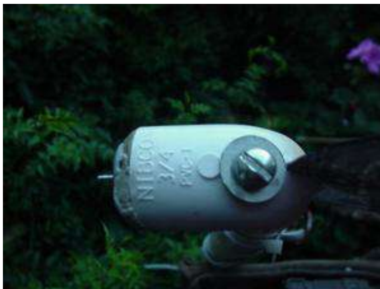
Top view showing yaw bearing bolt
