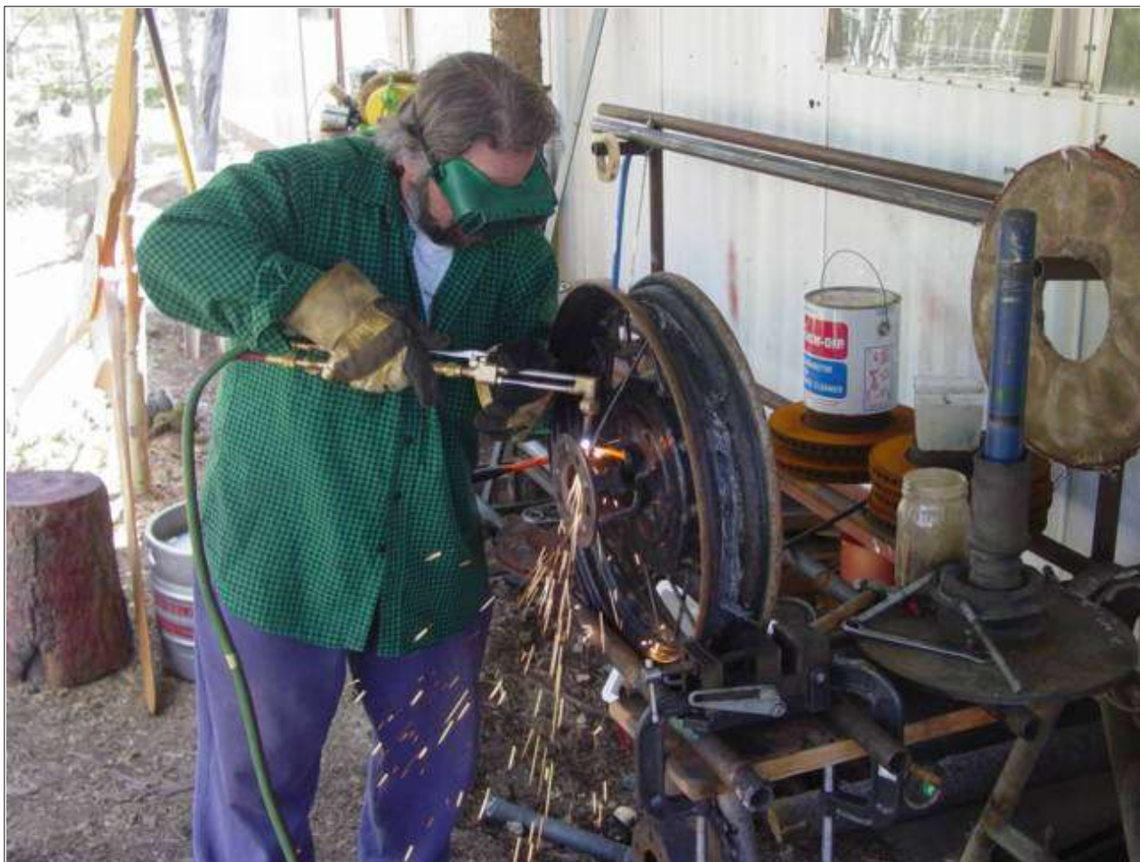
George was up and he helped me do some cutting and welding on an old warped/cracked wheel I had around.
