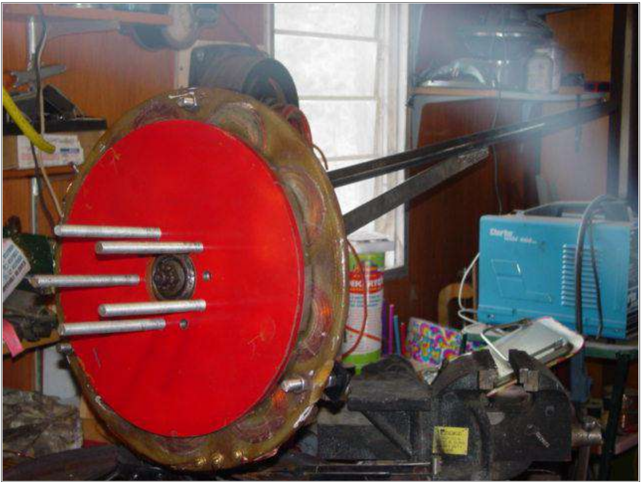
In this picture that alternator is finished, and we've fabricated the tail boom.
