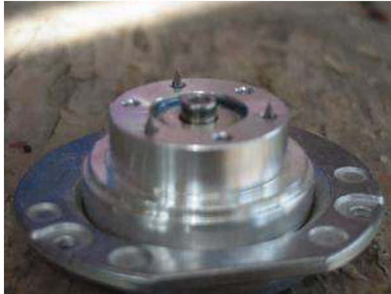
Nails in motor for marking hub holes.
