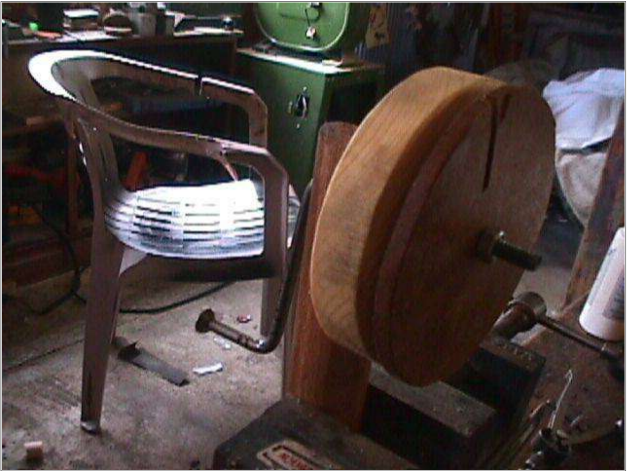
I made a simple hand cranked coil winder.
