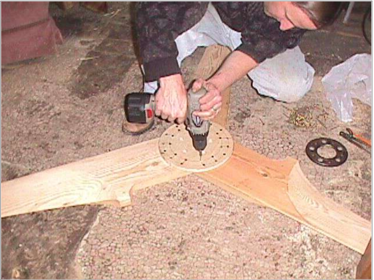
Here Scott is assembling the plywood hub that holds the blades together with 1.5" long wood screws.
