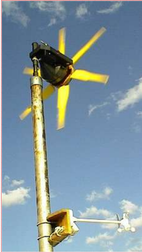
The downwind turbine, a very small but quite efficient little unit. This one was a bit more complicated to build but it features the star/delta controller ( check the link on downwind turbine for more detail)
