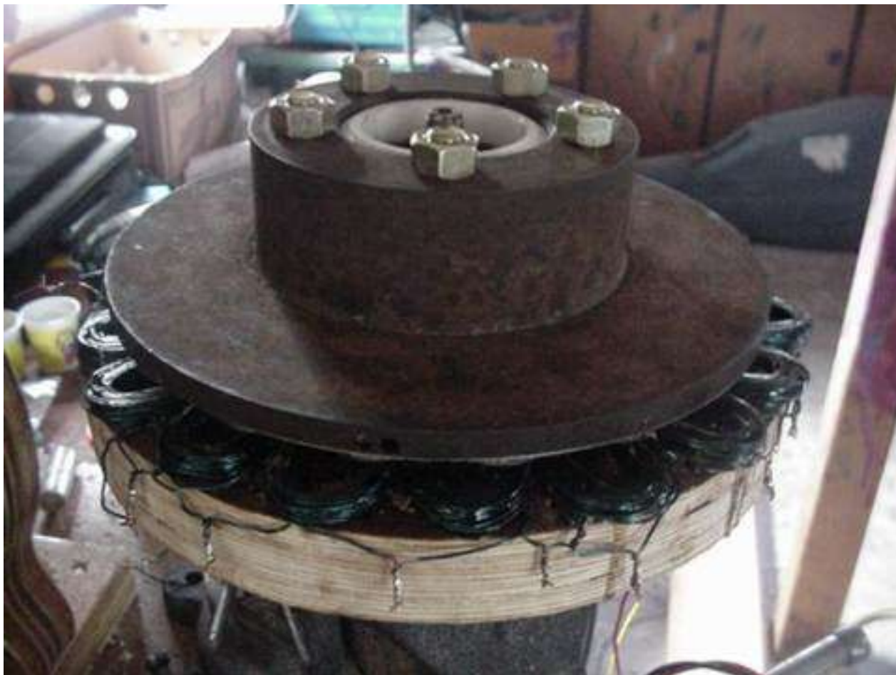
Homemade Volvo Brake Disc PM alternator, 800 watts, $150!
