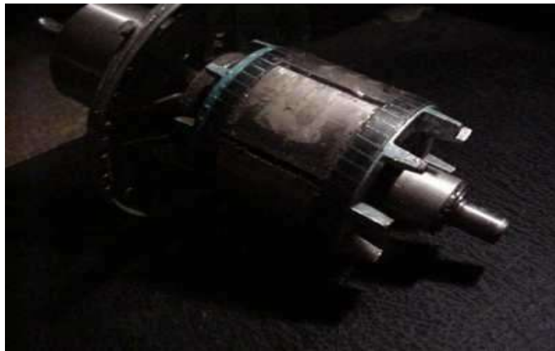
Armature converted with permanent magnets
