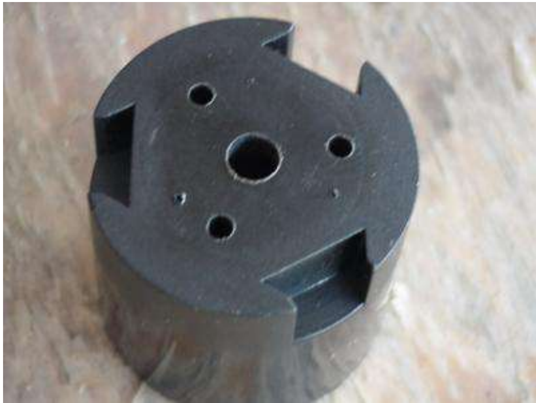
Completed anemometer hub assembly
