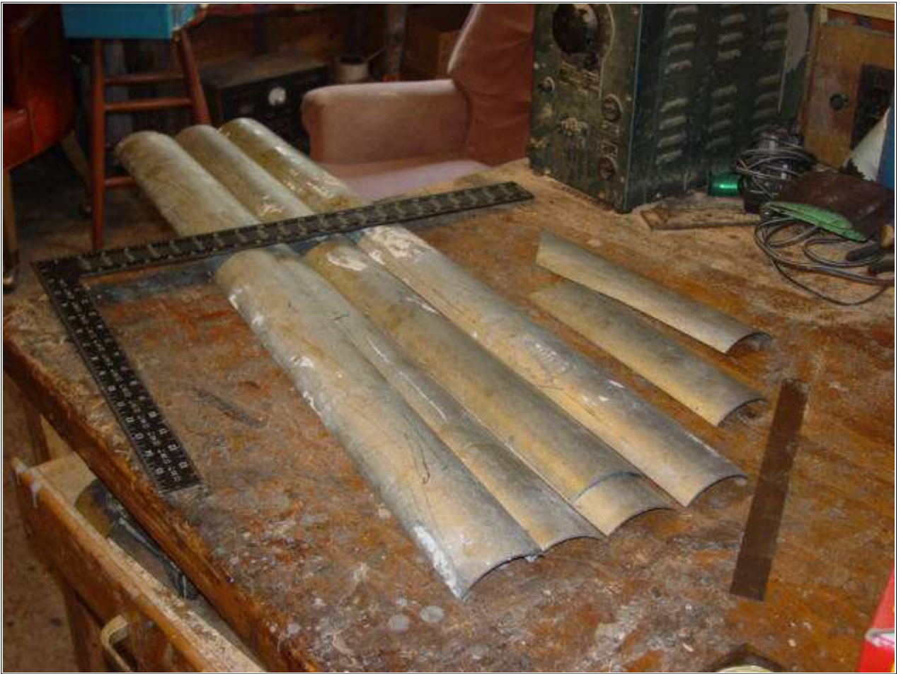
The Vanes in the runner are made from quartered 4" diameter steel conduit.
