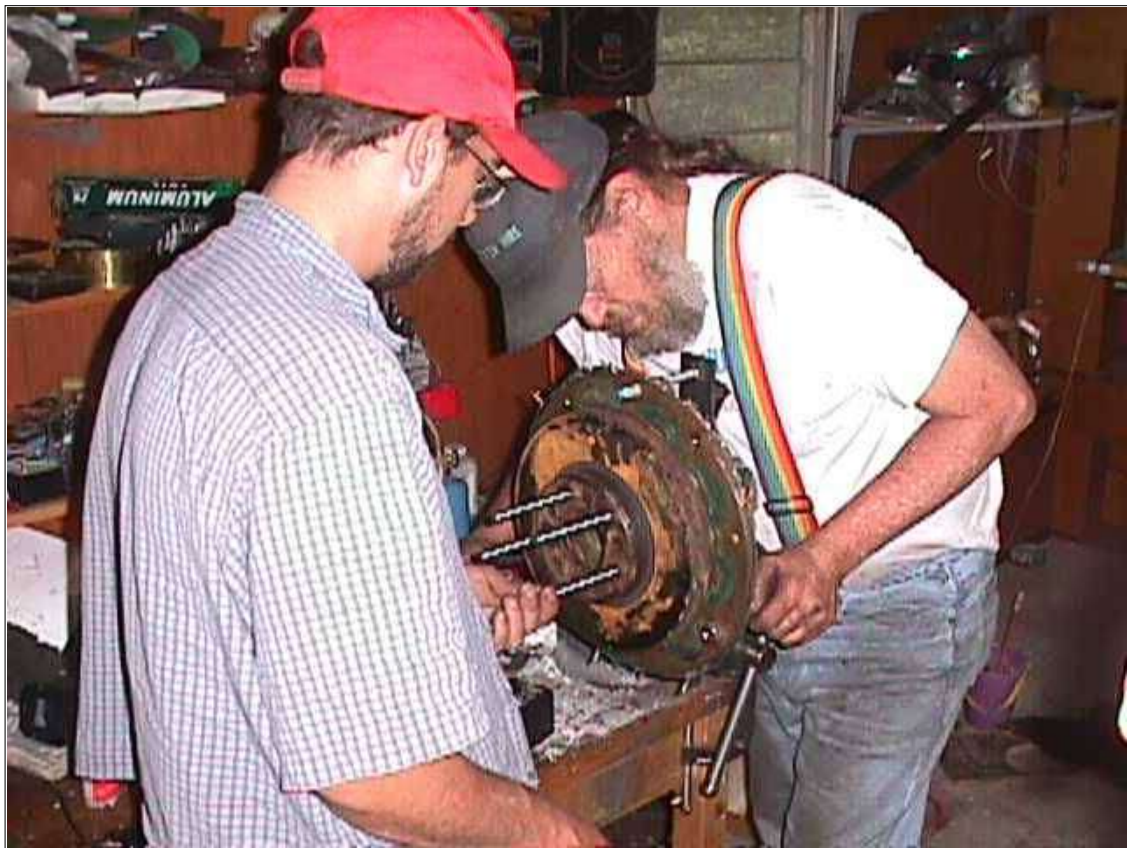
In the picture above we are hand turning the alternator and testing for output.
