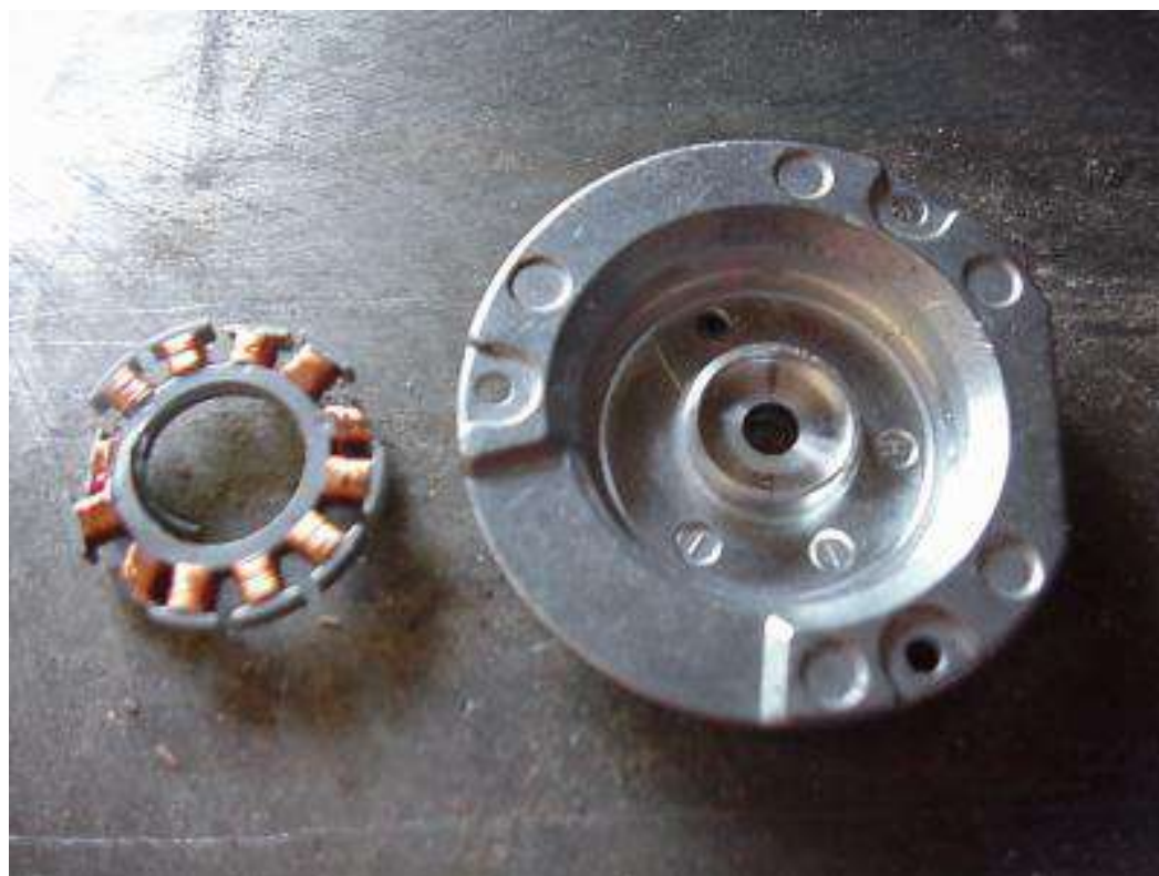
Coils removed from Motor
