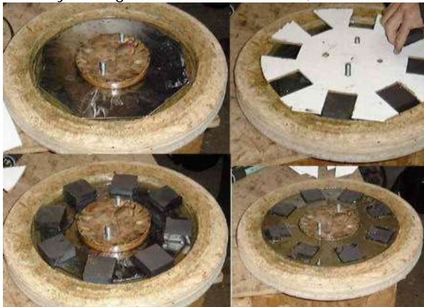
Four stages of the rotor casting procedure
