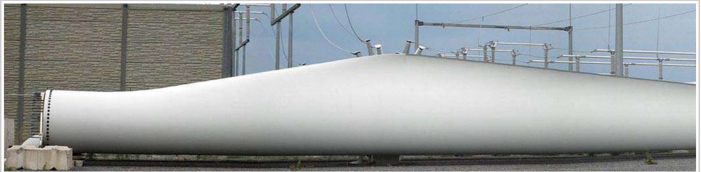
Fiberglass-reinforced epoxy blades of Siemens SWT-2.3-101 wind turbines. The blade size of 49 meters [40] is in comparison to a substation behind them at Wolfe Island Wind Farm.
