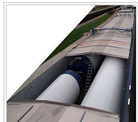
Sections of a wind turbine tower, transported in a bulk carrier ship
