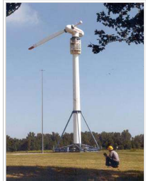
The NASA test of a one-bladed wind turbine rotor configuration at Plum Brook Station near Sandusky, Ohio
