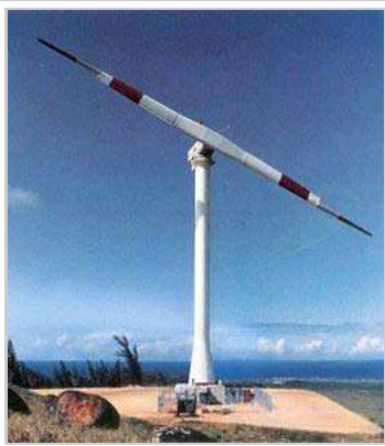
The 98 meter diameter, two-bladed NASA/DOE Mod-5B wind turbine was the largest operating wind turbine in the world in the early 1990s
