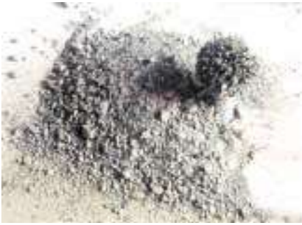
Magnetite sand collected from Dan's driveway by dragging a magnet around on a string.
