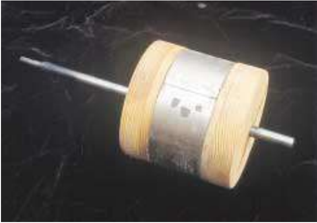
The wooden armature holds eight NdFeB (neodymium-iron-boron) magnets arranged in alternating polarity around its perimeter.
