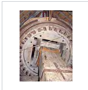
Windshaft, brake wheel, and brake blocks in smock mill d'Admiraal in Amsterdam
