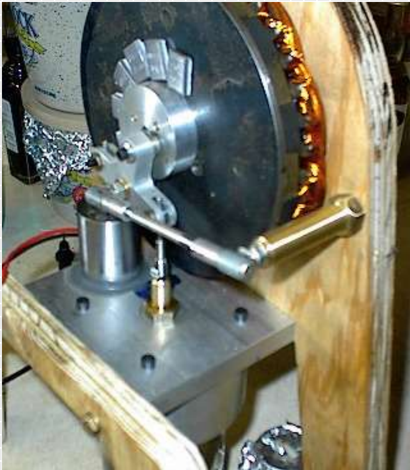
Above is another angle of the stabilizer rod to the yoke....
