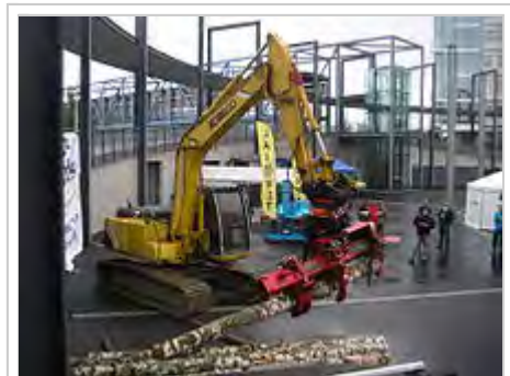
A Croco log splitter attached to a Kobelco excavator in Jyväskylä, Finland.
